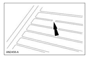
4. Using a polypropylene film fine line tape, mask the area directly above and below the grid break extending the tape 26 mm (1.02 in) beyond the concern area in both directions. The break area should be at the center of the mask.
