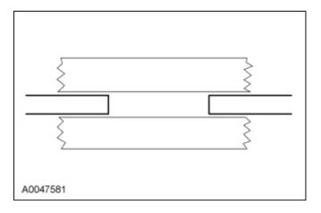
5. **NOTE:** If the brown layer is not broken or missing, apply only the silver grid repair compound to the break. If both the brown and silver layers of the grid are broken or missing, apply a coating of the lacquer touch up paint across the break in the grid line prior to applying the rear window defroster repair compound. Do not overlap the silver grid line with the paint. Several applications may be necessary to achieve a color match.
