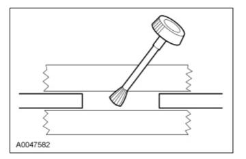
6. **NOTE:** The repair coating air-dries in approximately one minute and can be energized after 5 minutes. Optimum adhesion occurs after approximately 24 hours.
